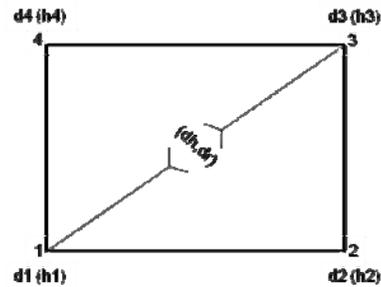
b. Rules proposed to put diagonal and horizontal distance measurements on the Filed Survey Form (Surat Ukur)
