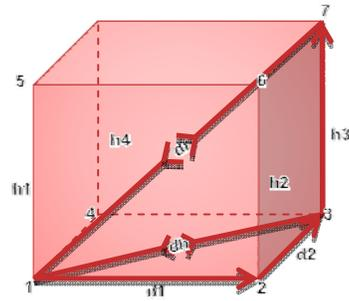
a. Illustration of measurement processes done to verify horizontal and diagonal distances of a registered apartment unit
