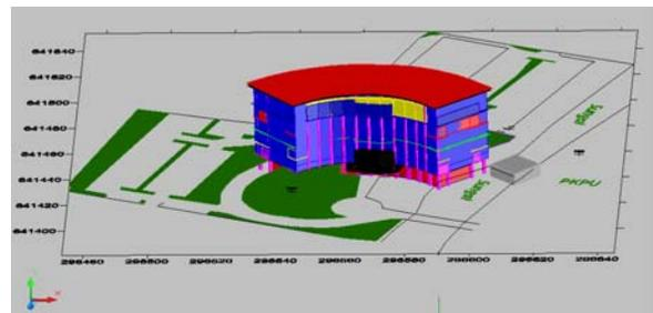
**Figure 3.** The resulted AutoCAD drawing of Postgraduate School Building of UGM generated from measurements of building outlines and floor plan.
