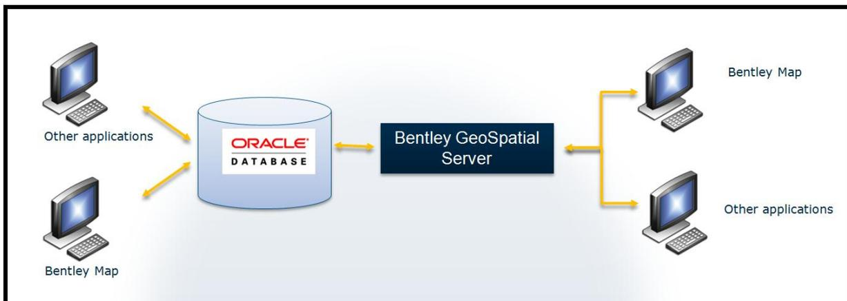
**Figure 9. Example of multi-tier architecture combining Oracle Spatial 11g and Bentley Geospatial Server to serve data to different desktop applications**
