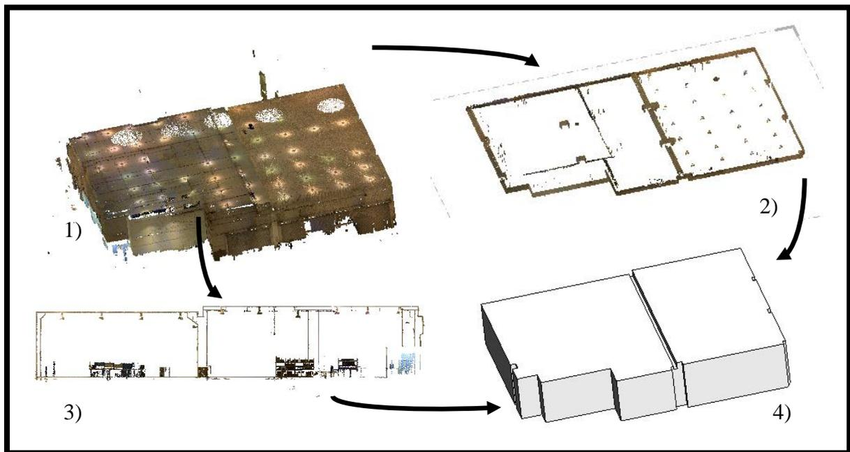
Figure 7. From Point Clouds (1) to Building Sections (2 and 3) to Solid geometry (4) (Point Cloud courtesy of Faro)
