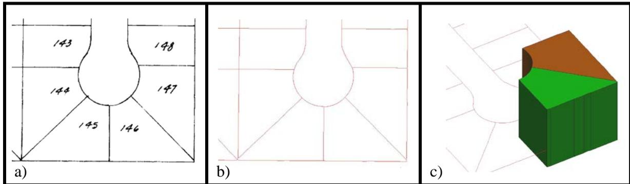
Figure 4. From 2D Raster (a) to 2D Vectors (b) to 3D Solids (c)
