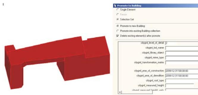
Figure 8. Create a 3D GIS object from polygons and attach properties
