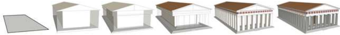
Figure 4. Illustration of the process of defining rules that iteratively refine a design by creating more and more detail. (Source: CityEngine help)
