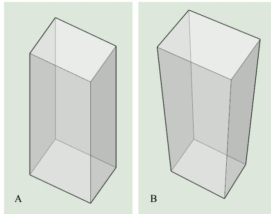
*Figure 2.3. Same 3D scene with different projection: A, orthographic projection; B, perspective projection*
