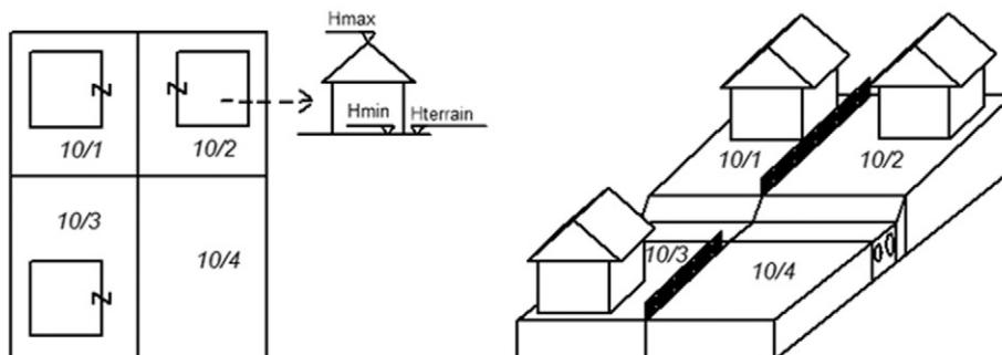
Fig. 7. The first case study: the current cadastral representation in the land cadastre and building cadastre (left), and the proposed 3D cadastre solution (right).
