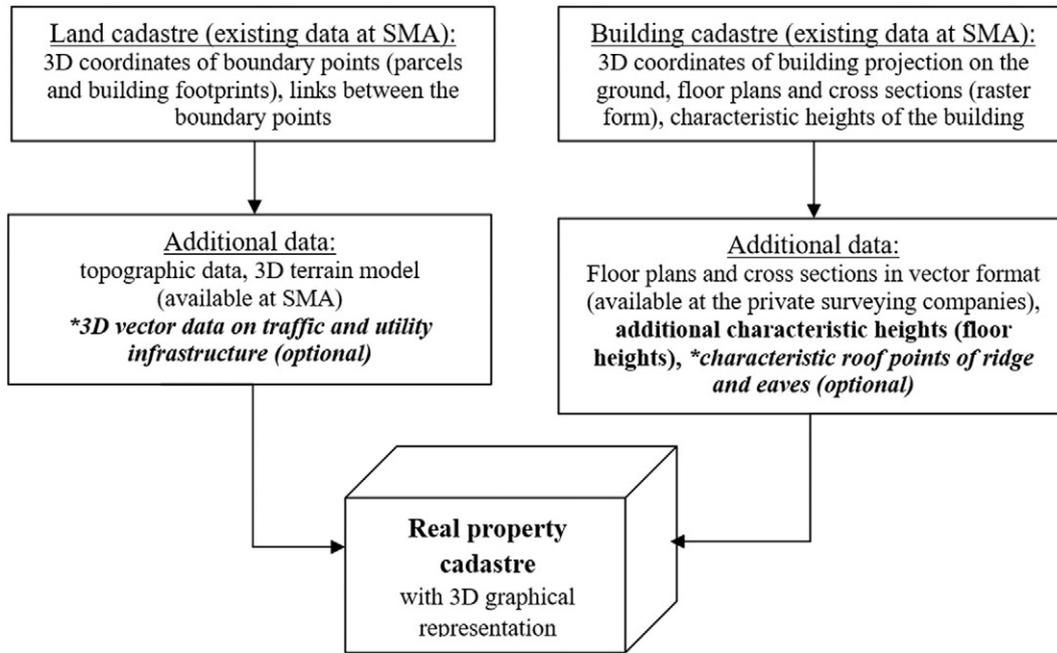
Fig. 6. Transition to a 3D real property cadastre in Slovenia by merging the land cadastre and the building cadastre – additional data required to establish the 3D cadastre with data representation in a 3D environment are outlined (data that are currently not available at the SMA or collected during the cadastral procedure are shown bold).
