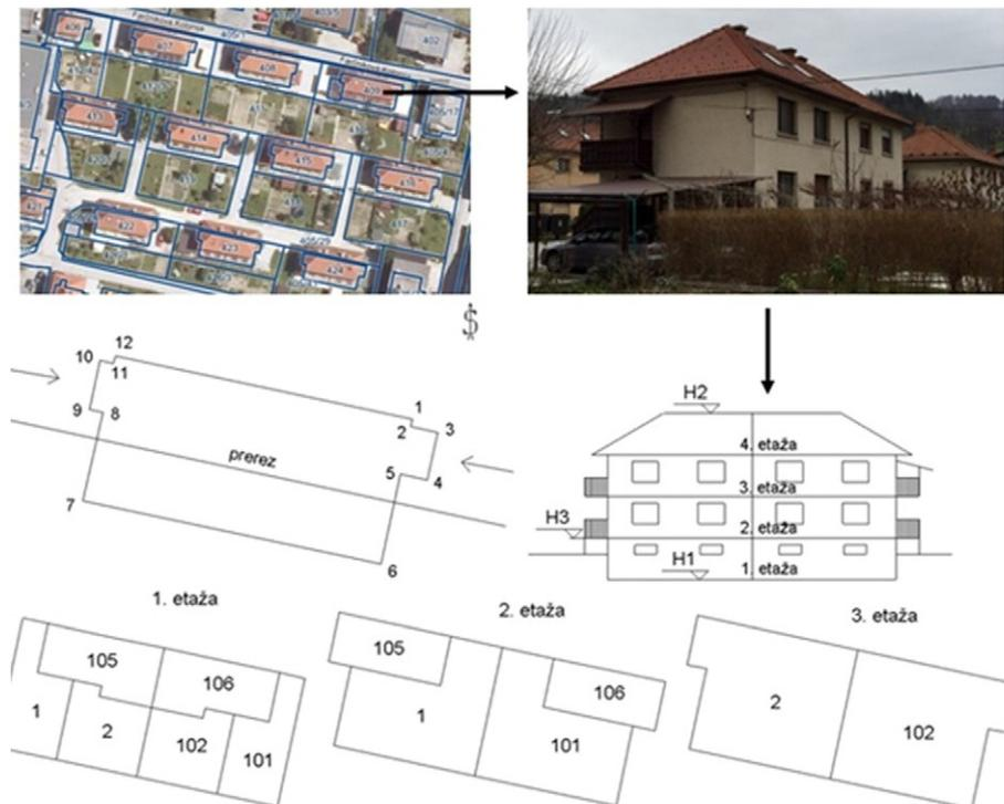
Fig. 10. A land cadastre map with land parcels and buildings' footprints on orthophoto (upper left corner), and graphical representation of the selected building in the building cadastre (the projection of the building to the ground, vertical section with characteristic heights, and floor plans).
