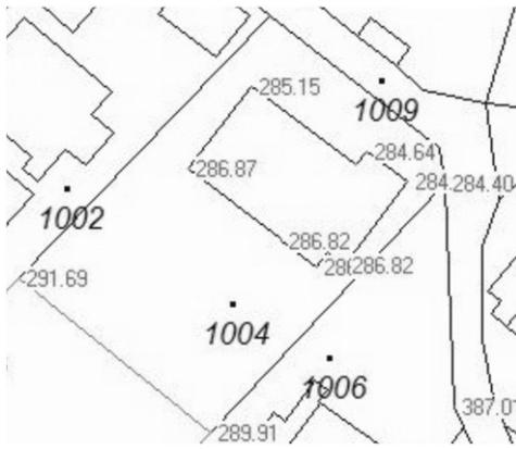
**Fig. 4.** Graphical representation of vector data in the land cadastre – the building's footprint on parcel 1004 is linked to the building in the building cadastre. (Source: Surveying and Mapping Authority of the Republic of Slovenia).
