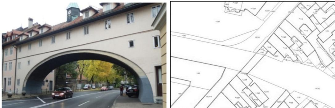
Fig. 1. In the Slovenian cadastral system, a building can be graphically represented on the cadastral maps in a 2D environment (thicker lines) as a projection of the building on the ground. (Source of cadastral data: Surveying and Mapping Authority of the Republic of Slovenia).
