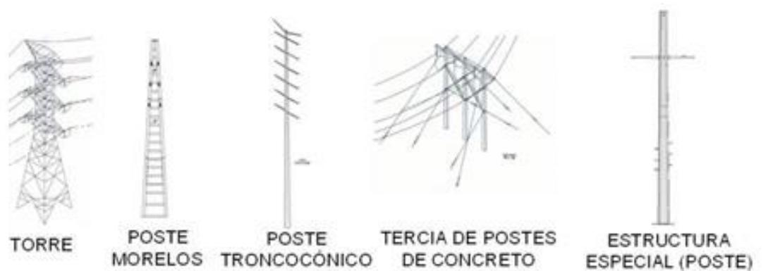
Figure 3. Typical support structures for transmission lines in Mexico
