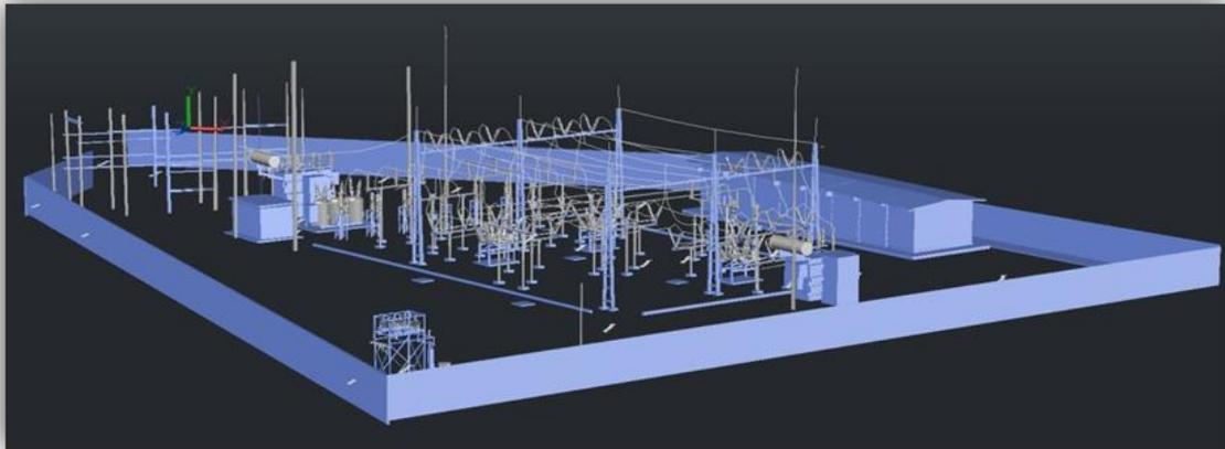
**Figure 7. Representation of the site of a substation surveyed with Total Station and terrestrial scanner**
