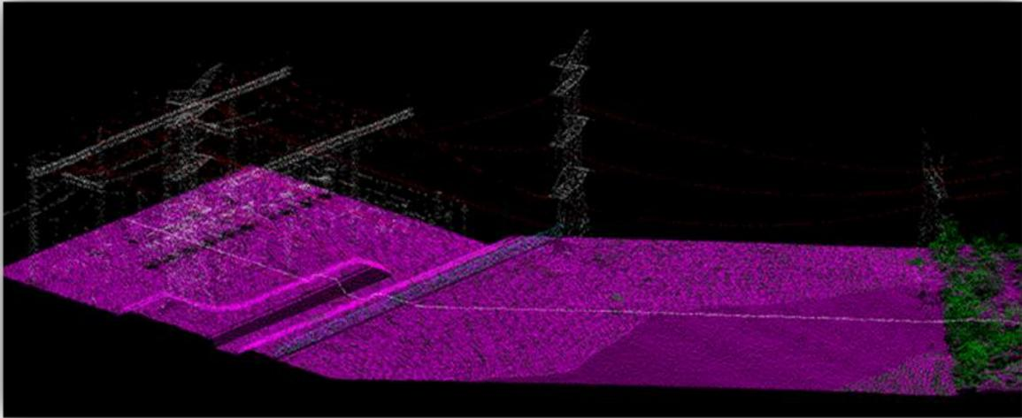
**Figure 8. Representation of the site of an existing substation, surveyed with LiDAR**
