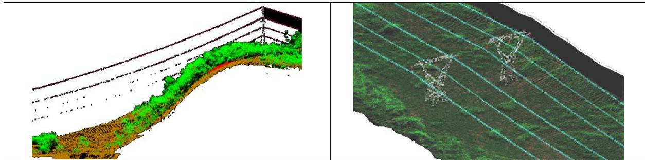
**Figure 12. Representation of the transmission lines from LiDAR data**
