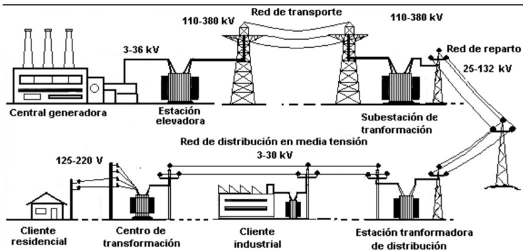
**Figure 2. Power substations and Transmission Lines**
