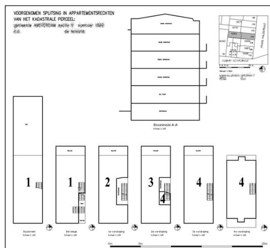
**Figure 1. Example of a drawing (“splitsingstekening”) of the apartment complex. The boundaries of the private parts are in thick black lines.**
