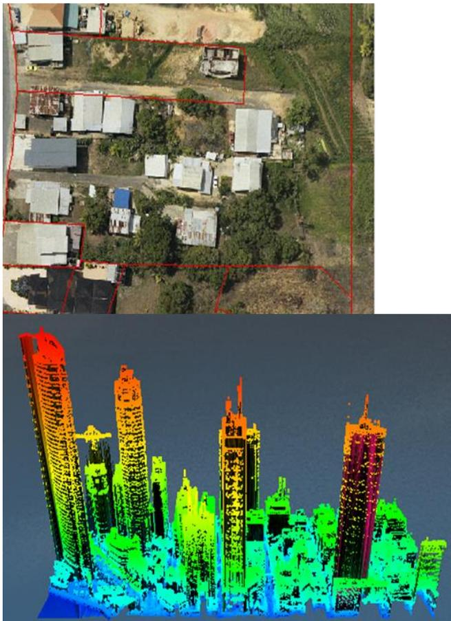
**Figure 12 (a) Orthophotography indicates topography related to the cadaster (b) LiDAR data of urban Trinidad and Tobago**
