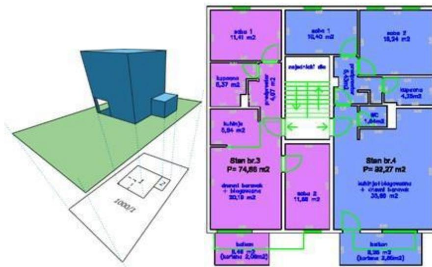
**Figure 3. Property on the cadastral map and presentation of parts (separate and common) per floor**
