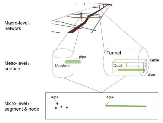
**Figure 9.** Multilevel structure of utility networks.
