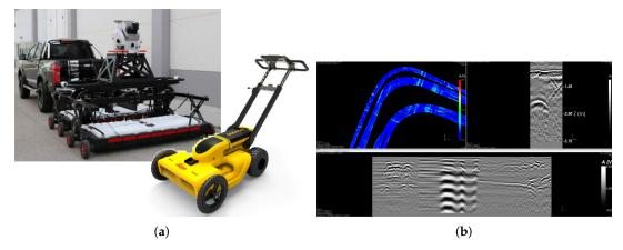
**Figure 4.** Examples of **GPR** instruments (a) and **GPR** data (b); the data show a radargram of a longitudinal cross section of the top-most about 2.85 m along an asphalt paved road (bottom), a perpendicular cross section of one lane (top right) and the top view of the scanning tracks covered by GPR measurements (top left).
