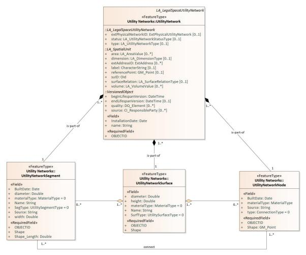
Figure 10. The classes diagram of utility networks.
