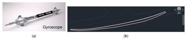
**Figure 5.** An example of a gyroscope-based pipeline measurement system (**a**) and the 3D map of the measured pipes (**b**).
