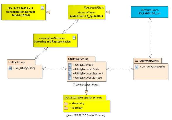
Figure 8. The overview of packages of the 3D underground utility data model.
