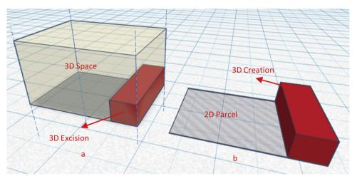
Fig. 21. a) Excision of volumetric space, b) creation of a volumetric lot (Source: (Karki et al., 2013)).
