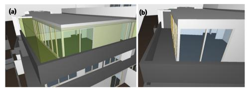
Fig. 18. Two representation of (a) legal space (watertight), (b) physical boundary (non-watertight).
