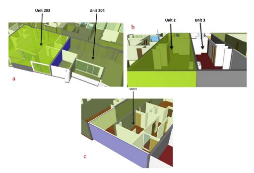
Fig. 28. 3D visual representation of building boundaries, a) Interior boundary, b) Median boundary, c) Exterior boundary (Source: (Atazadeh et al., 2017)).
