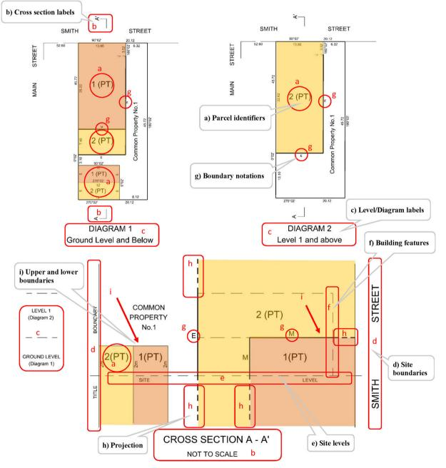
Fig. 11. A snapshot of what must be checked in a 2D floor plan and cross section.
