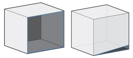
Fig. 17. Two non-watertight 3D samples; a) missing face b) the gap in the surface.
