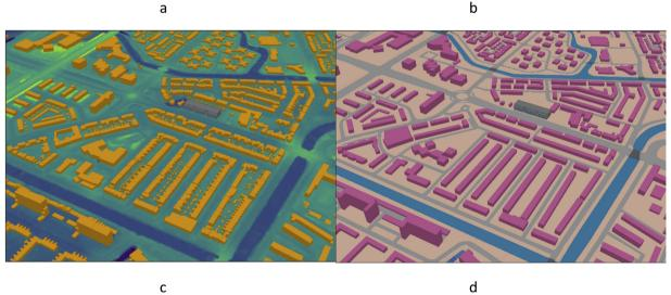
Fig. 4. Obstacle models (a) Model 1: DSM produced with first return points of AHN3 (b) Model 2.1: DTM plus buildings with rooftop geometry (c) Model 2.2: DTM plus buildings extruded with mean height of rooftop point (d) Model 3: TOP10NL dataset.
