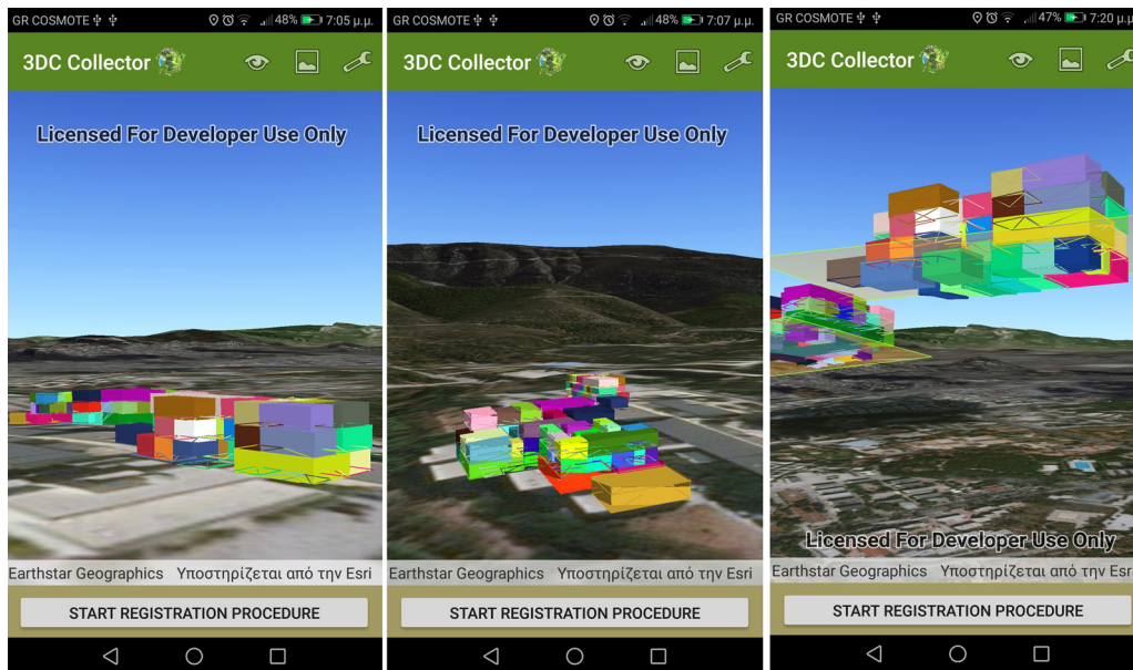
Fig. 16. 3D models of the declared properties above (left, middle) as well as above and below (right) the ground, using the 3D Model tool of the developed mobile application.
