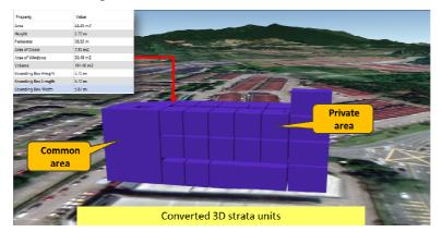
**Figure 6: The strata units based on the integration of BIM model and Strata XML.** In this method, the flexibility of IFC as a standard for BIM was utilised to harness the rich data for the conversion such as *IfcSpace* and *IfcZone* as source elements suitable for 3D
