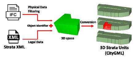
Figure 1: The overall of data integration from IFC model and Strata XML into 3D Strata Unit.
