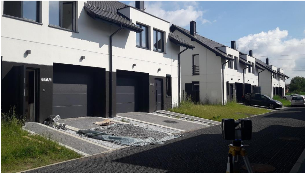
Figure 7. TLS instrument Faro Focus X310 during point cloud acquisition
