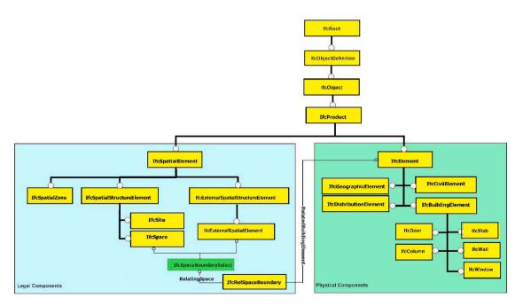
Fig. 5. Different sections of the IFC standard used for modelling legal and physical components.
