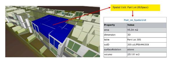
Fig. 7. A typical spatial unit (building unit) modelled in the BIM environment.
