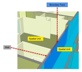
Fig. 12. An example of boundary line passing through the centreline of a wall.
