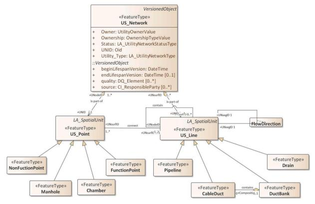
Fig. 4. The Utility Core package.
