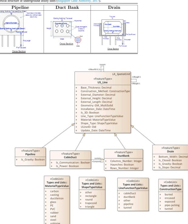
Fig. 6. The US\_Line class and its subclasses.
