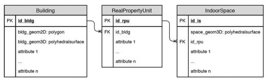
Figure 9 DBMS implementation of the proposed cadastral data model
