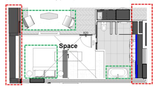
**Figure 8.** Duplicated floor system limiting space boundaries and causing gaps and overabundance of geometrical information highlighted by the green dash.
