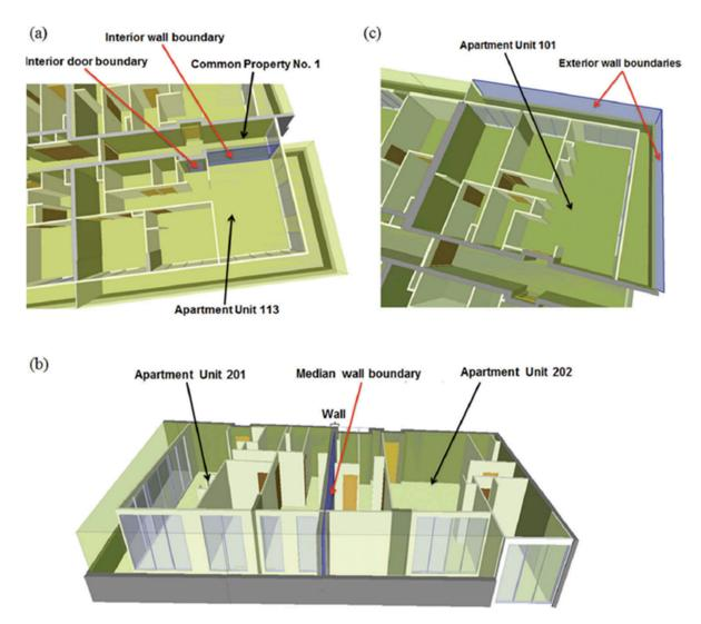
**Figure 2.** Various boundary locations. (**a**) Interior, (**b**) Median, (**c**) Exterior, Reprinted with permission from [36]. 2016 Behnam Atazadeh.
