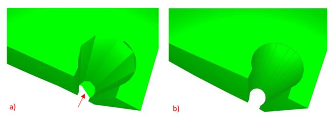
Figure 12. Errors in the data transformation stage. (a) An invalid IfcSpace, (b) a valid IfcSpace.
