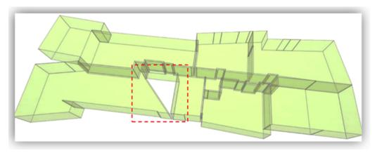
**Figure 10.** Errors in authoring cadastral information stage. An undefined ownership space due to incorrect modelling leads to a gap created in the IFC data format.
