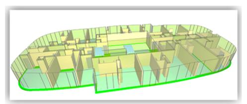
Figure 6. A slab (in green) representing common property as one object.
