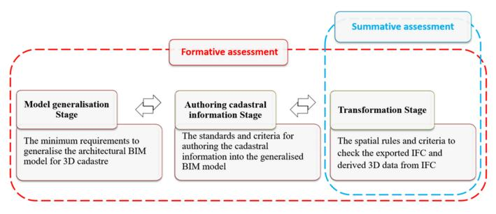
Figure 15. A formative and summative assessment to check the spatial consistency and integrity of BIM-based cadastral data.
