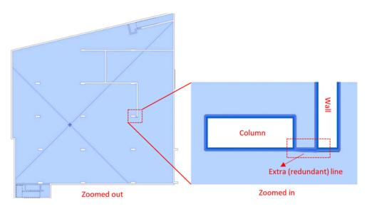
Figure 20. Detected error in the model generalisation and transformation stage.
