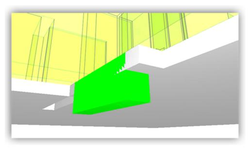
Figure 7. Hard clash detection in physical objects.
