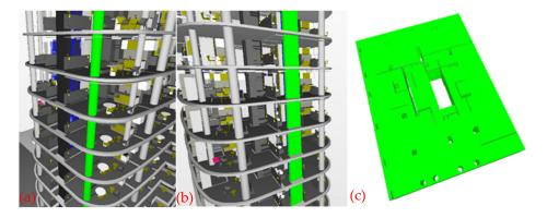
**Figure 5.** (a) Non-floor-specific design of columns and (b) shear walls as one object; (c) A non-simple polyhedron representing a slab caused by non-floor-specific design of column.
