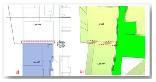
**Figure 9.** Errors in authoring the cadastral information stage. (**a**) An undefined ownership space in the BIM model, (**b**) a gap created in IFC data format.
