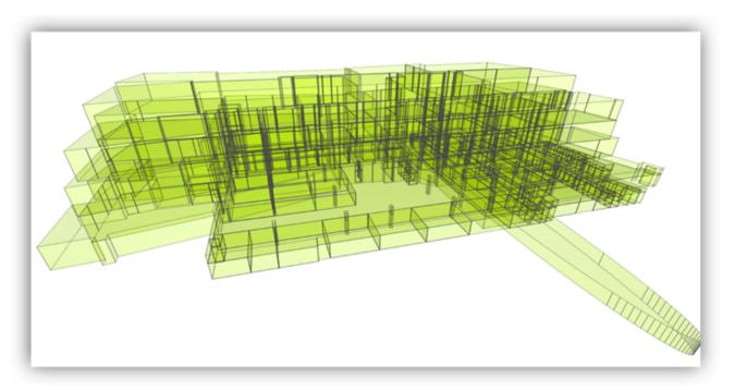
Figure 16. IfcSpaces representing volumetric legal spaces exported from enriched BIM model.
