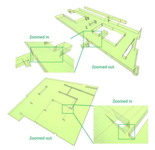
Figure 22. The rectified IfcSpaces after implementing the formative assessment.
