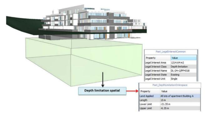
Figure 3. Leveraging BIM for 3D representation of depth limitation. Reprinted with permission from [15]. © 2016 Behnam Atazadeh.
