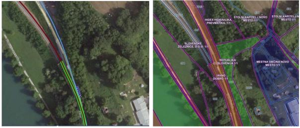
Figure 12. Left: railway (red) with the tunnel (green) and road (blue); right: the land plot and ownership structure (Source: PISO, https://www.geoprostor.net/piso)
