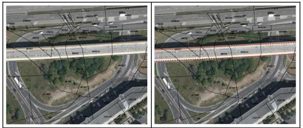
Figure 7. Even if a part of the line B is located inside the outdoor tunnel, it is not reflected on the cadastral map (left). Here in the figure the outdoor tunnel is highlighted with red dashed line (right)
