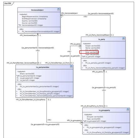
Figure 3. Additional Primary key has been created for each table (Alattas et al., 2018)
