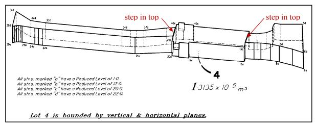
Figure 4. This spatial unit can fairly readily be decomposed into a "footprint" of vertical walls, and well defined sets of faces defining the top and bottom
