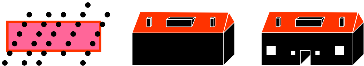
Figure 30 Building object in 2D, overlaid with denser laser data (left). The more laser points, the more details can be reconstructed (middle and right).
