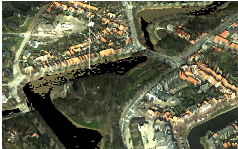
Illustration 3: TIN terrain rendering for Middelburg (AHN data). Notice that sharp features (e.g, buildings,trees) are not well captured by the TIN.
