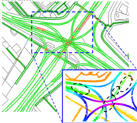
Figure 6. Standard deviations of map point heights. Compare with available laser points (lower right corner).
