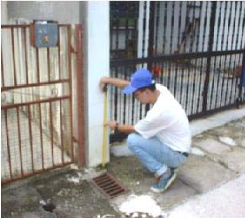
a. Flood mark measurement after the flood event
