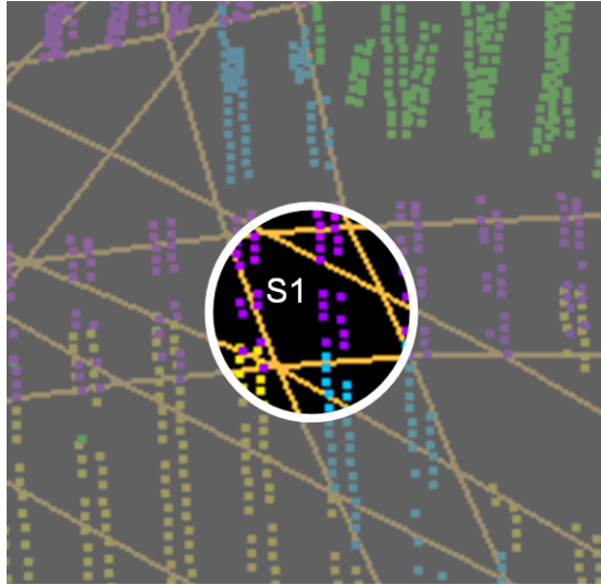
Figure 9 Situation 1 (S1) This polygon should be modelled at three different heights, but only contains laser points on the highest level, and one laser point on the intermediate level, and no one the lowest level.
