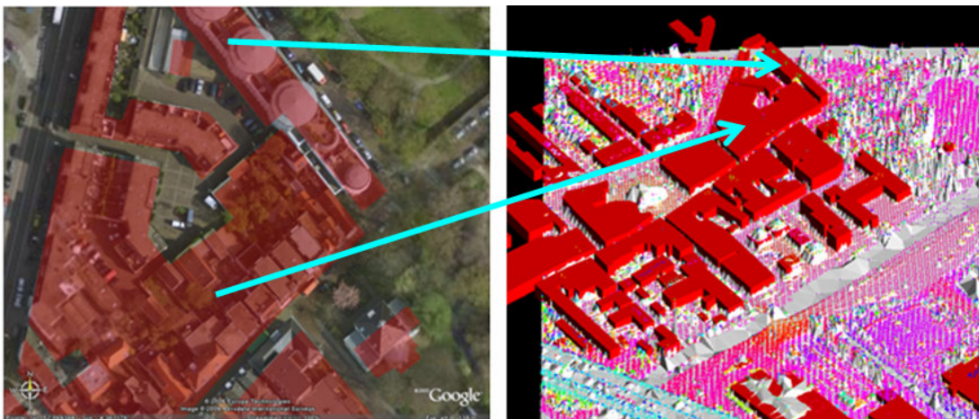
Figure 4 Building polygons overlaid on image (left), blocks of buildings displayed with laser points (right).
