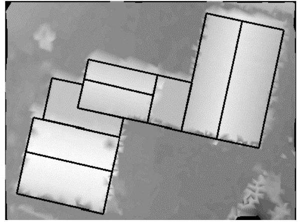
Figure 11 Final partitioning after merging segments assigned to the same planar faces.
