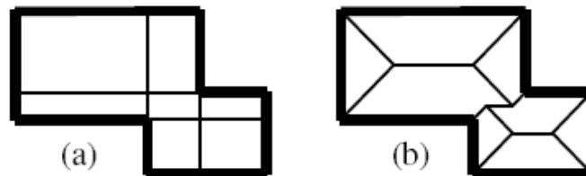
Figure 32 Segmentations of ground plan by (a) extension of lines at concave corners or (b) intersecting planes through the eaves, assuming horizontal eaves at one height and the same slope for all roof faces (source [Vosselman, 2002]).
