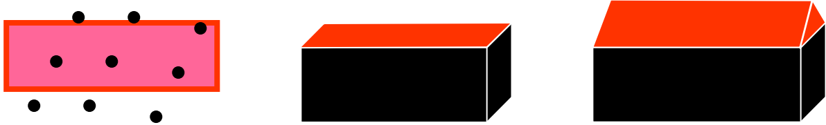
Figure 29 Building object in 2D, overlaid with laser points (left). Two possible shapes in 3D: flat roof (middle) and gable roof (right).
