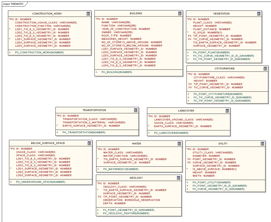
Figure 3: Spatial schema of the semantic tables in alternative I (Emgård and Zlatanova, 2008b)
