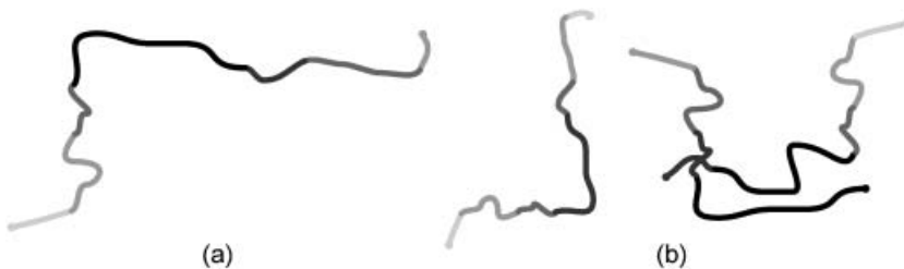
Figure 7. Vague line objects: (a) a vague line and (b) a vague multiline.
