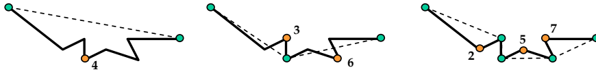
Figure 6. Three steps of Douglas-Peucker algorithm for edge simplification. The edge is drawn in thick black line; edge approximation on each step is drawn in thin dashed line. Vertices in green are part of the approximation; in orange are vertices selected for inclusion in the next approximation.
