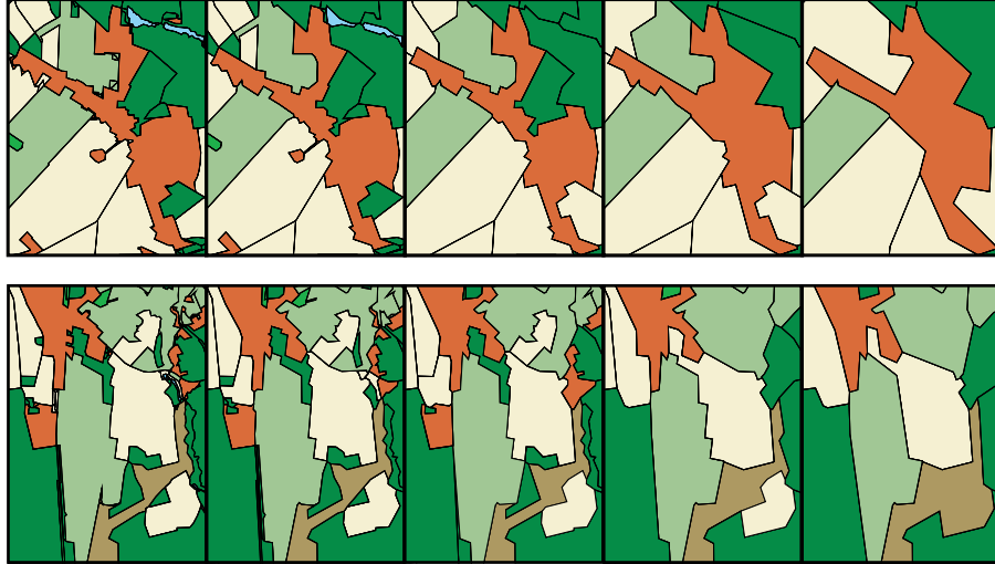
Figure 7: Two examples processed with Algorithm 1. From left to right: most detailed dataset with additional boundaries S_{\text{overlay}} , found intermediate representations, and dataset generalised by optimisation S_{\text{lowLoD}} .
