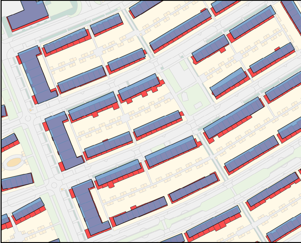
Figure 6: IMGeo buildings (in red) overlaid with Top10NL buildings blocks (in blue). The background is IMGeo data that is made transparent.
