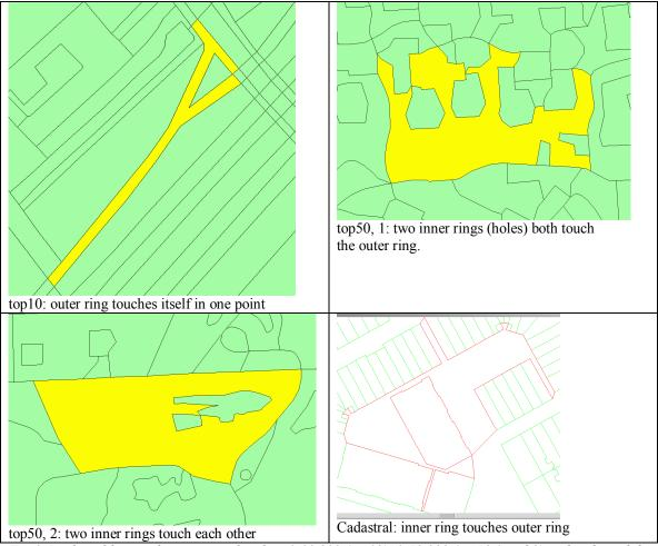
Fig 1. Real world examples: topographic data 1:10.000 (top10), 1:50.000 (top50 1 and 2) and cadastral data.
