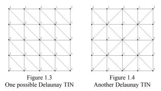
In Figure 1.3 the diagonal of all triangles is directed north-west to south-east. The four points on a square are on the same circle, so it is with the Delaunay criterion in mind, free to choose a direction for the diagonals, as there is no optimum for the min-max angle criterion. This could be north-east to southwest for all diagonals, more or less data dependent distributed as in Figure 1.4 or even complete randomly distributed. Which one to choose?
