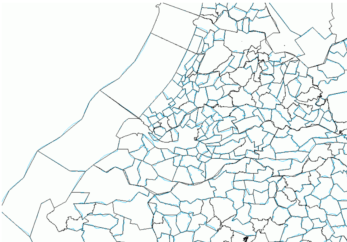
Figure 3.5. Effects of BLG-tree generalization on data. Original data in blue, generalized data in black.
