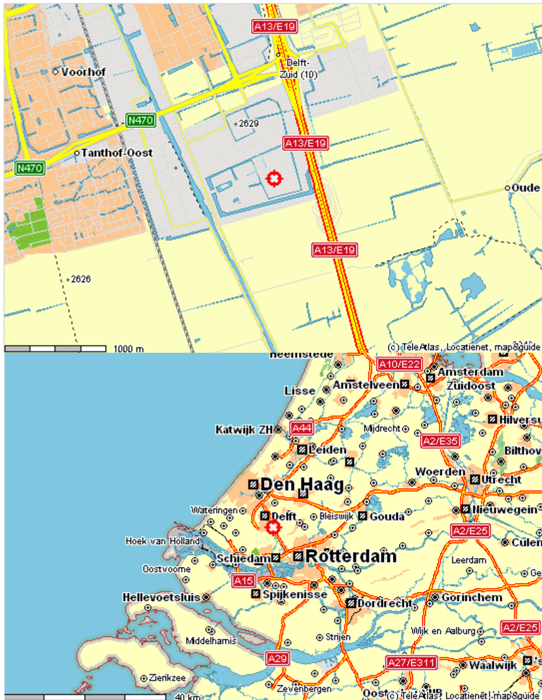
Figure 2.1: Example of need for generalization. Lower image would be totally cluttered if the detail level of the upper map was used.[24]
