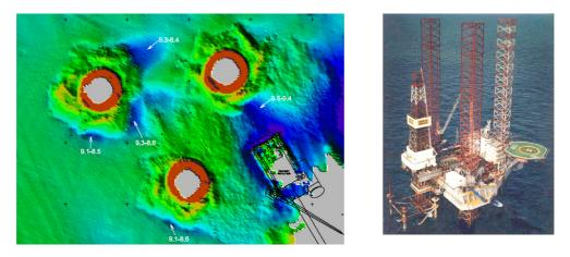
Figure 1: Bathymetry impression of jack-up rig footprints (up to 15 metres deep).
