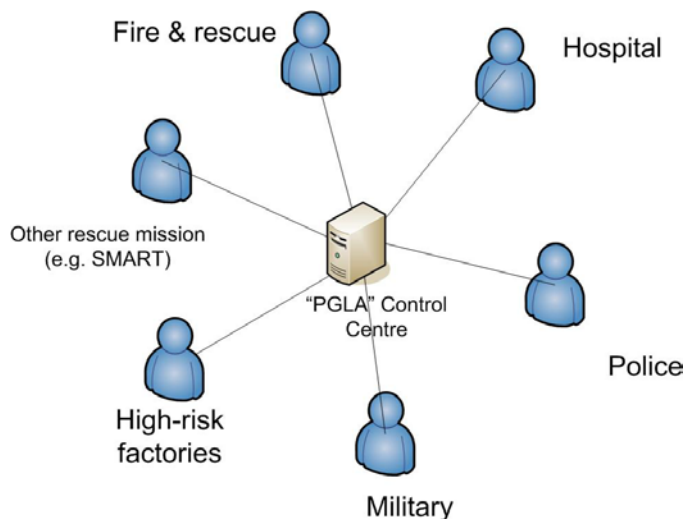
Figure 4: The system architecture for the “Pasir Gudang” Local Authority (PGLA) control centre.
