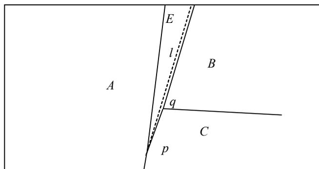
**Figure 8-15 Polygon point *q* has been inserted into line *l*.**
