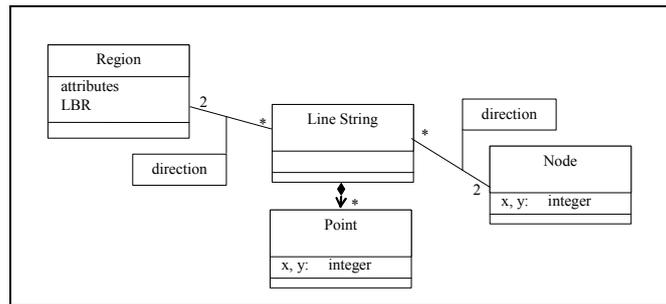
Figure VII-6 a 2D polygonal region with topological encoding.
