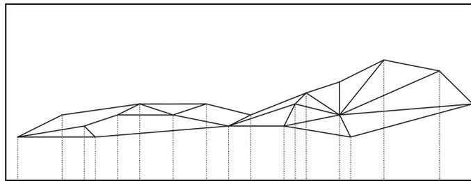
**Figure 10-1 A regular polytope used to define a land surface topography. The convex polytopes are delineated with solid lines to show their upper surface and dashed lines to delineate their vertical faces. They have no lower faces, being unbounded below.**
