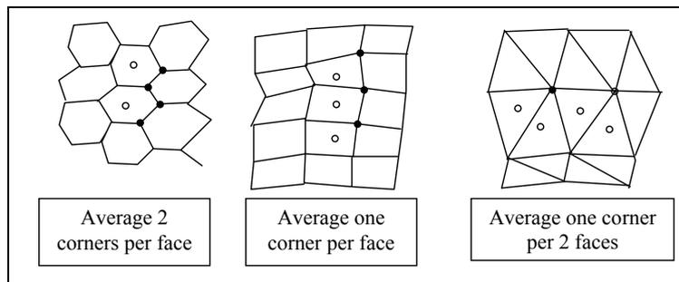
Figure VII-2 Ratio of corners to surface patches.
