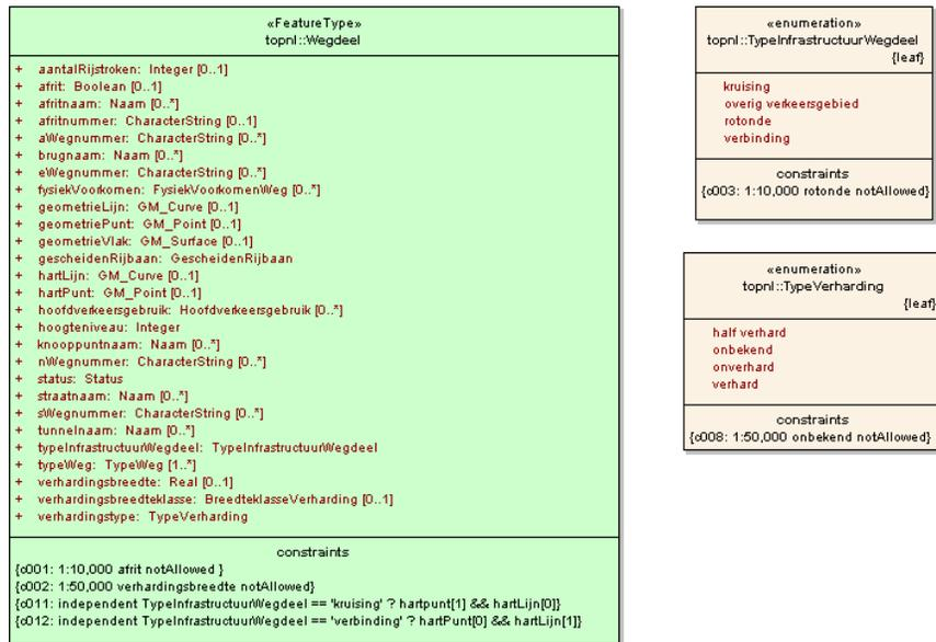
**Fig 3:** Using constraints to model scale dependent information (inheritance from GeoObject is not shown)
