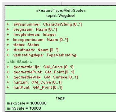
**Fig 5:** Example of using a MultiScale stereotype to model scale dependent information
