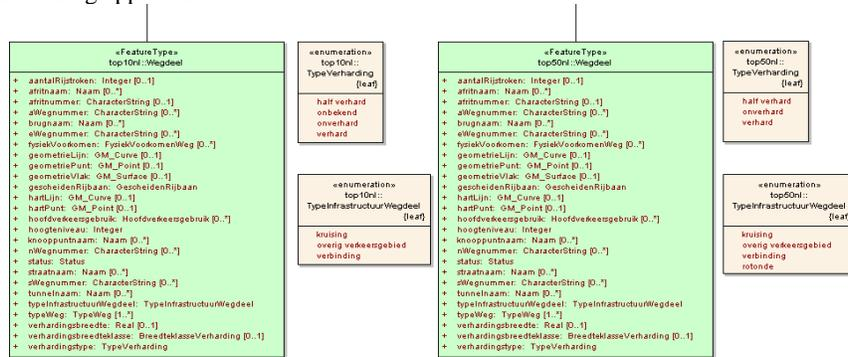
Fig 2: Separate UML class diagram per scale (inheritance from GeoObject is not shown)
