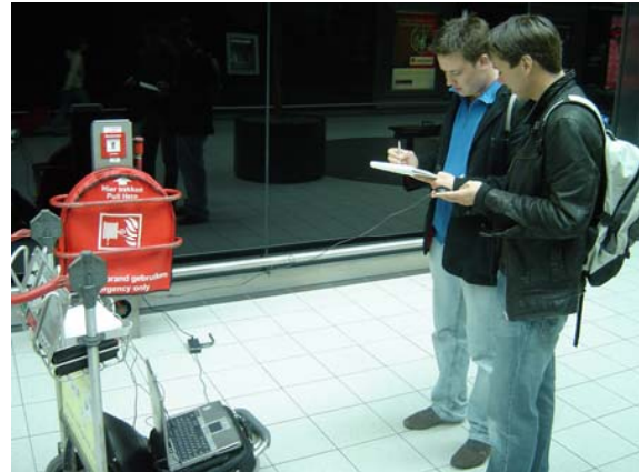
Fig. 2. Luggage trolley with u-blox receiver connected to a laptop, while the external (patch) antenna is held in hand.
