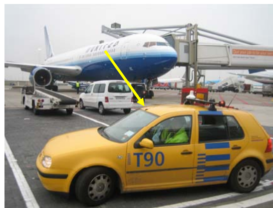
Fig. 8. Car used in Schiphol HSGPS outdoor test. The u-blox patch antenna is fixed to the roof of the car (see arrow).
