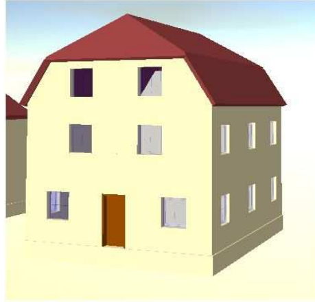
Fig.5: Geometrical Representation of a building in CityGML LOD 3 (CityGML Dataset, Four Buildings in LOD 3)
