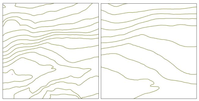
This is taken from 1:2500 data (classification O), omitting all contours and index contours with an elevation not divisible by 2m.
