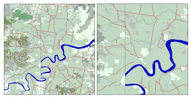
This level is also generalised from 1:250k data, by removing smaller area features, shorter linear features, and a random selection of point features. Note the break in the Brisbane River – the break can be seen here to be caused by missing small segments rather than an edge mis-join.
