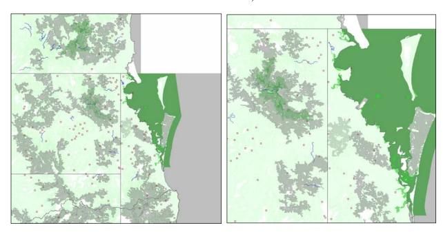
This level is generalised from 1:250k data, by removing smaller area features, shorter linear features, and a random selection of point features. Note that rivers have broken up into random segments. This would not have happened if they had been named or strung together as single features.
