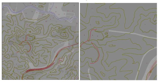
This has been taken from 1:25k data, omitting all contours and index contours that are not divisible by 10m.
