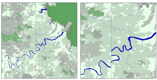
This level is also generalised from 1:250k data, by removing smaller area features, shorter linear features, and a random selection of point features. Note the break in the Brisbane River. The break can be seen here to be caused by missing small segments rather than an edge mis-join.
