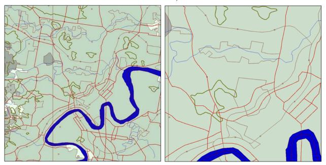
This is unedited 1:250k data. It was also used as the source for the levels E to H. Note the bight of the river that was removed form the smaller scale data – in particular, compare with level H.
