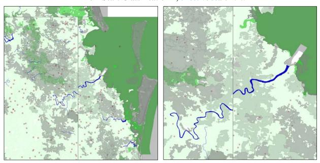
This level is also generalised from 1:250k data, by removing smaller area features, shorter linear features, and a random selection of point features. Note the break in the Brisbane River – This is an artefact of the area feature being broken at a sheet boundary in the data. Again, this will be corrected automatically when the feature is named.
