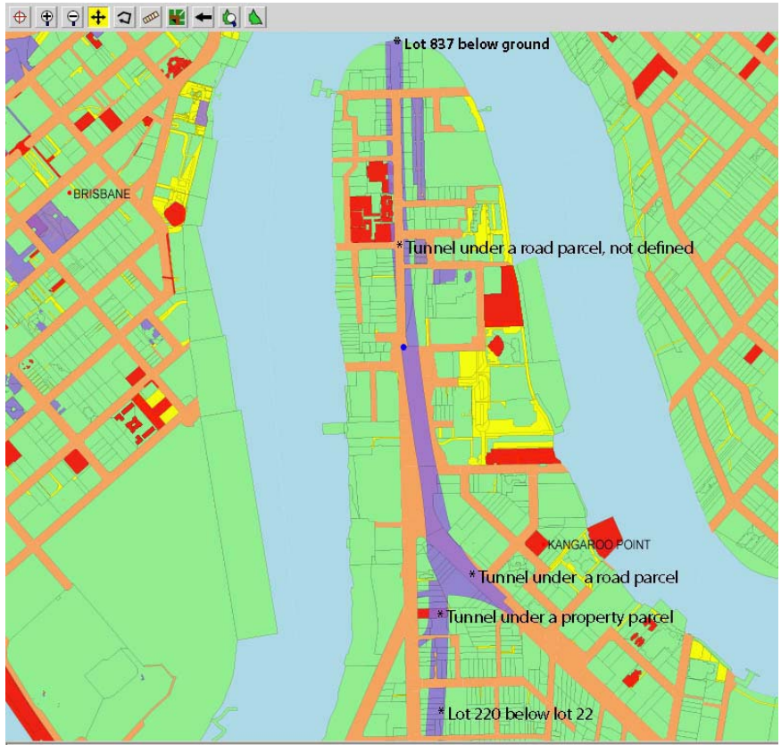
Figure 1 Tunnel running under surface parcels
