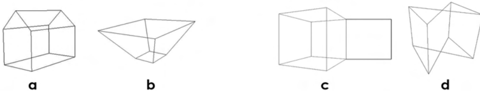
Figure 6-13 Examples of valid (a and b) and invalid (c and d) 3D objects.
