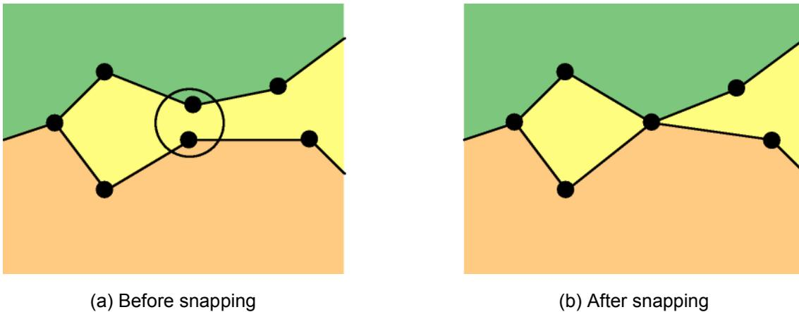
Figure 4: Polygons can be split by snapping, since some parts might be narrower than the threshold (encircled). While this result does not create an invalid result, it can change the number of polygons present and their topological relations, and can therefore be undesirable.
