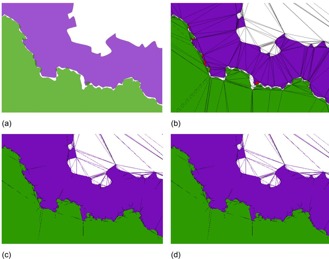
Figure 6: **(a)** Original dataset with two polygons. Notice the gaps (white) and the overlaps (darker green). **(b)** The CT of the input polygons; white triangles have no label, and red ones have  $>1$ . **(c)** Triangles are re-tagged such that each triangle has one and only one label. **(d)** The resulting edge-matched polygons.
