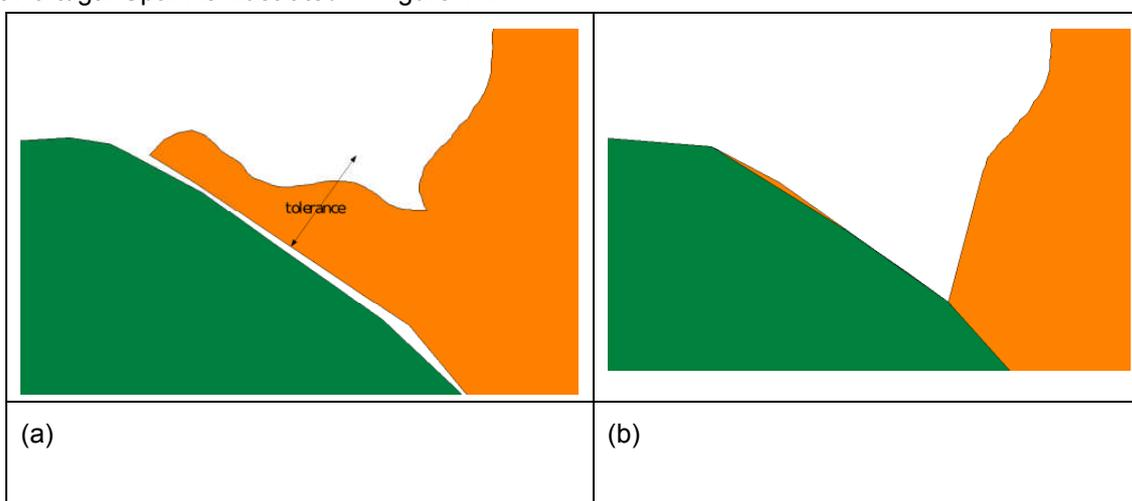
Figure 11: **(a)** Original dataset, with the tolerance used for snapping. **(b)** Collapsing of part of an polygon.
