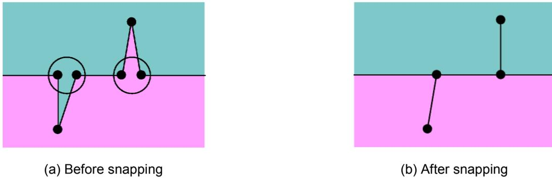
Figure 3: Spikes and punctures can be created by snapping, since the bases of these elongated forms (encircled) might be narrower than the threshold, but their lengths not.
