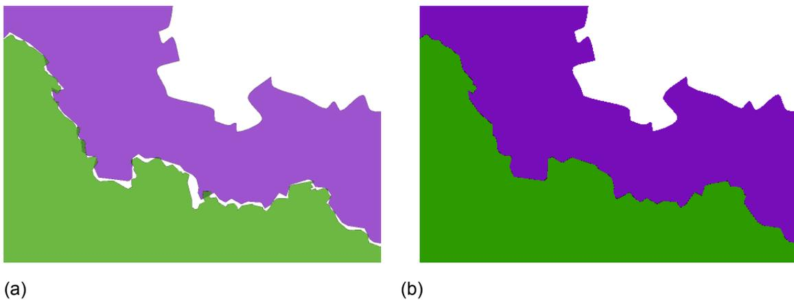
Figure 9: **(a)** The same dataset as Figure 6. **(b)** Edge-matching performed with a repair operation where the label assigned to a problematic region is the one of the adjacent neighbour having the longest common boundary. Notice the differences with Figure 6(d).
