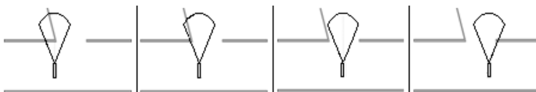
Figure 4. As a sensor moves along a corridor next to an open door, it detects the frame until no part of it is inside the area covered by the sensor.
