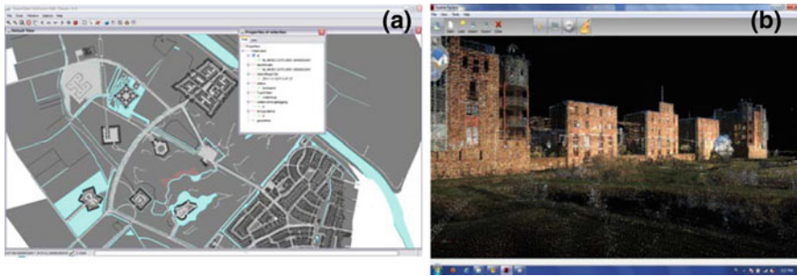
Fig. 4 Example source data available for the 3D Pilot test area. a 2D IMGeo data. b High resolution laser data, obtained by terrestrial laser scanning
