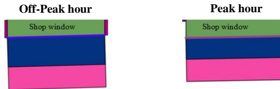
Figure 3. Functional area (blue and pink) of a shop (green) during off-peak (2 meters) and peak (1,5 meters) hours. Pink colour represents areas determined by the private space criterion.
