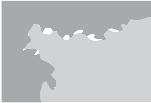
**Figure 23.** Alternative application of `SPLITAREA`: horizontal conflation. Two cross-border data sets have gaps (white areas) between them. `SPLITAREA` can be used to split those gaps. Figure taken from Ledoux and Arroyo Ohori (2011).
