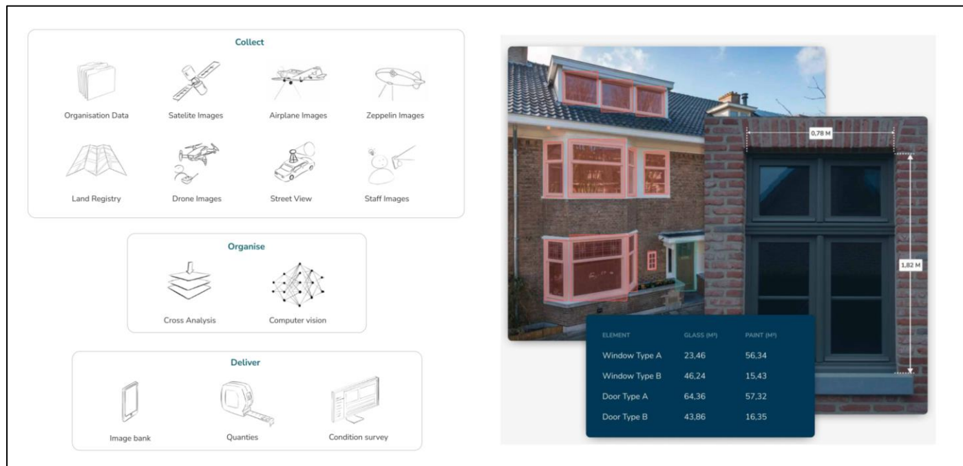
Figure 95: Image Indicating the overview of the condition assessment process using P advanced surveying techniques. Source: Modified from content received from facadeserviceapplicatie.nl
